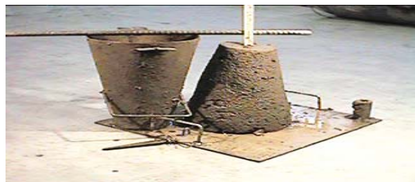
Consistenza S1: slump 0 - 40 mm
