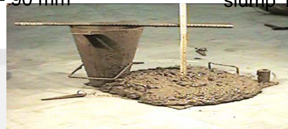
Consistenza S5: slump > 210 mm
